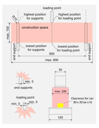
The supports and the loading points contacts have to be rigid parts of the bridge (e.g. not prestressed elements).
