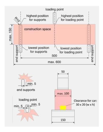
The supports and the loading points contacts have to be rigid parts of the bridge (e.g. not prestressed cords or similar).
